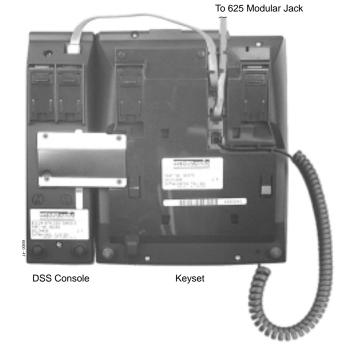
Figure 4-6 INSTALLING A 110-BUTTON DSS CONSOLE
