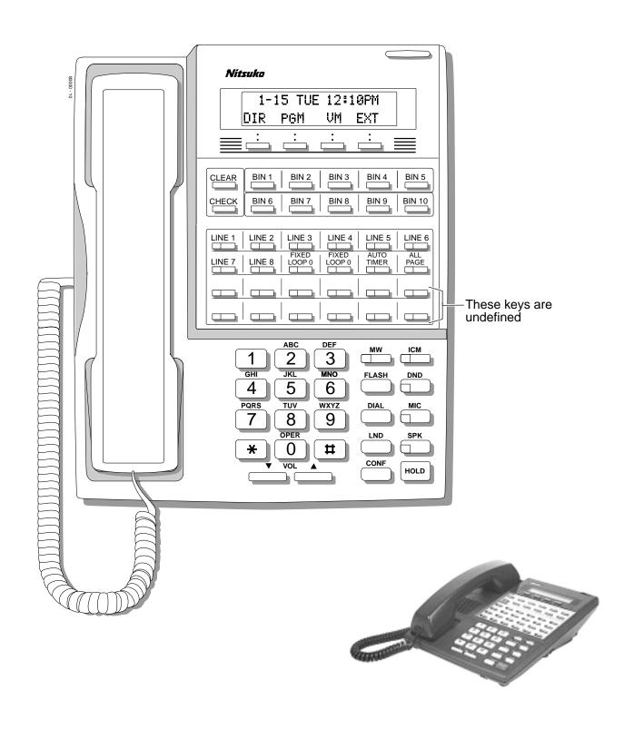
Figure 3: 34-Button Display Telephone
