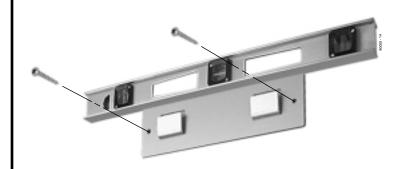
Figure 1-4 MOUNTING THE WALL MOUNT BRACKET
