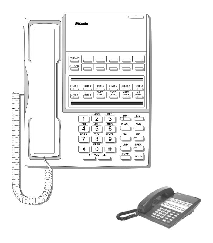
Figure 2: 22-Button Standard Telephone
